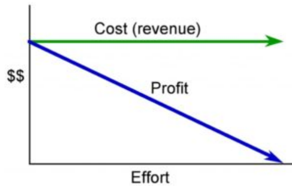
Figure 13.1: In a fixed-price contract, the cost to the client is constant regardless of effort applied or delivery date.
